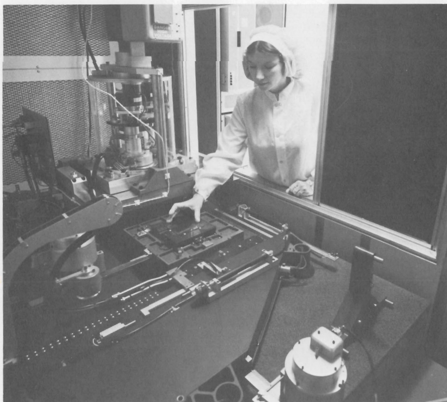
At Santa Clara Division, Susette Urmeneta loads a photomask "camera" or pattern generator that photographically draws a miniaturized version of an IC design, under the direction of a computer. This equipment has replaced the large copy cameras that once made photo reductions for ICs that were far simpler than today's.
