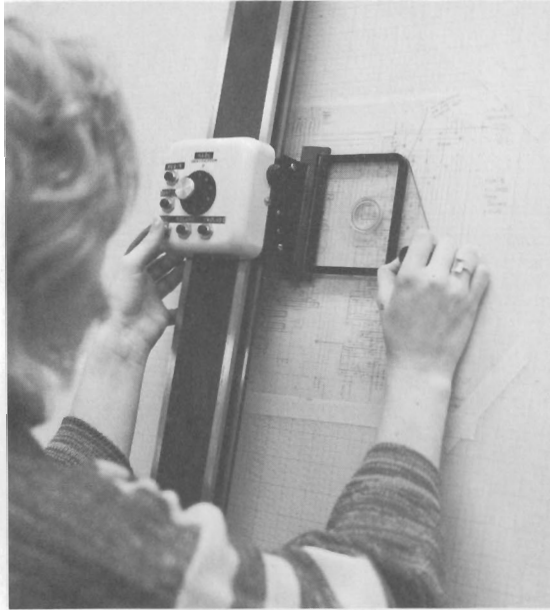
Sandi Carr of Data Systems Division "digitizes" a sketch of a new integrated circuit design and enters it into the computer. Much of the software used in IC design and production was developed within the company.
